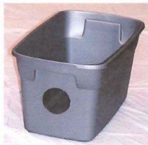
Cut 5 1/2" diameter hole in tote
